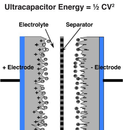
Figure 5: Ultracapacitor Structure Diagram
