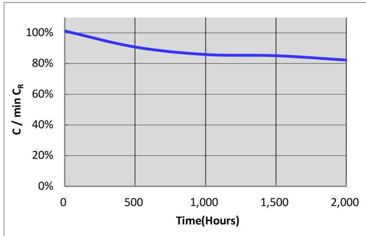
Figure 3: Accelerated Aging Capacitance Performance
