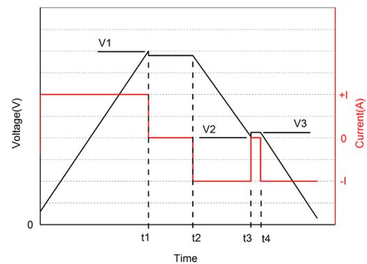
Figure 2: DC-ESR Measurement Waveform
