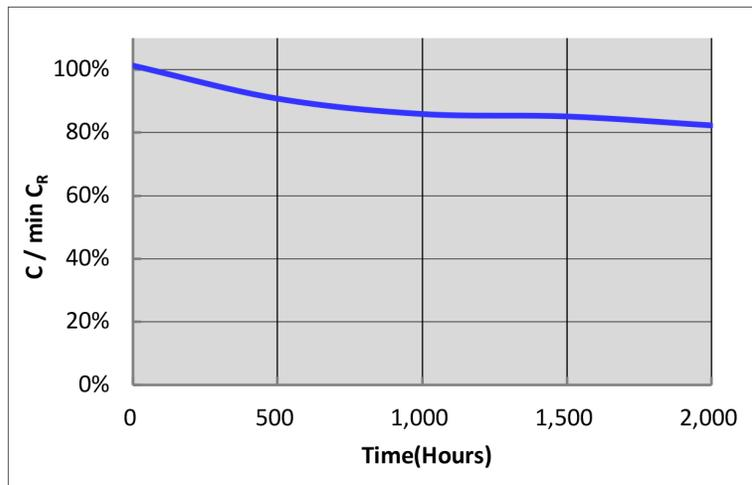
Figure 3: Accelerated Aging Capacitance Performance
