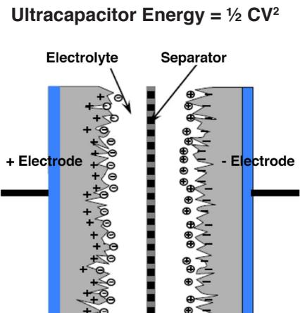
Figure 5: Ultracapacitor Structure Diagram
