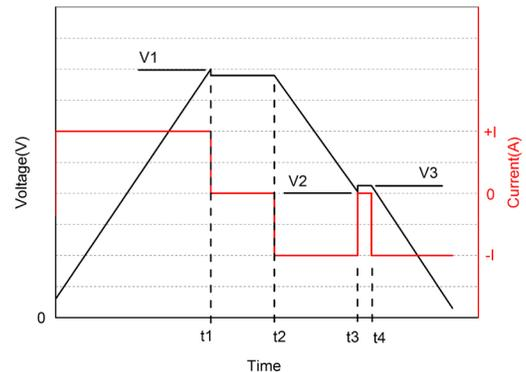
Figure 2: DC-ESR Measurement Waveform
