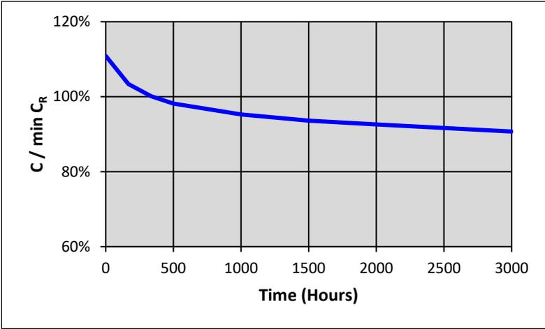
Figure 3: Accelerated Aging Capacitance Performance
