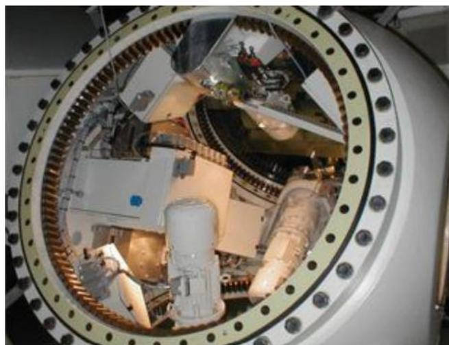
Figure 1 Independent electromechanical pitch actuators
